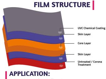
Film is designed for UV off set sheet printing in box lamination
